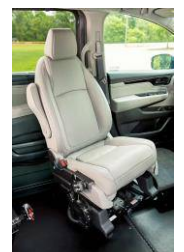
Swivel-style car seats can come out of the car or turn inside of the car. 13,14
