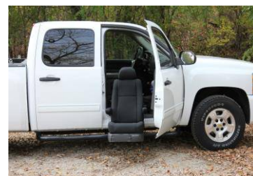
Swivel-style car seats can come out of the car or turn inside of the car. 13,14
