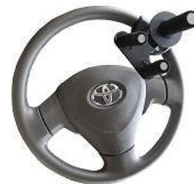
A spinner knob can be used to increase control when driving. 17
