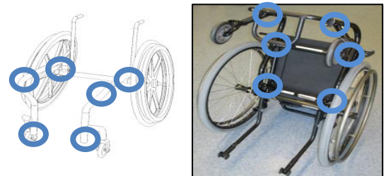
Common sites of nuts and bolts on manual wheelchairs. 23
