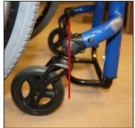
Caster stem that is not aligned with the caster wheel. 19
