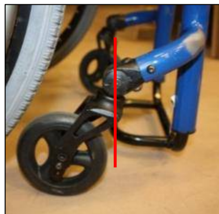
Caster stem that is not aligned with the caster wheel. 19
