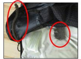
Cover foam liner flaking 14
