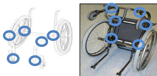
Common sites of nuts and bolts on manual wheelchairs. 23
