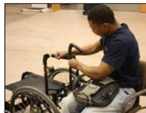
Inspect back posts and back support hardware
