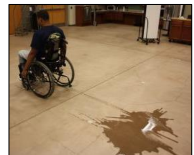
One way to check tracking is by rolling through a puddle of water. Take note of the water trail made from the wheels. Are they parallel and straight? 32
