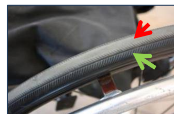
Intact (green) and worn out (red) tread on a wheelchair tire. 15
