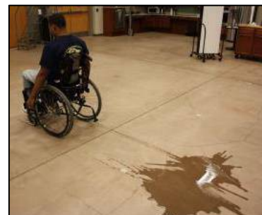
One way to check tracking is by rolling through a puddle of water. Take note of the water trail made from the wheels. Are they parallel and straight? 32
