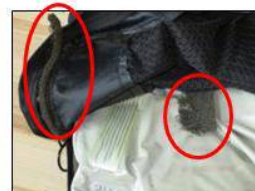
Cover foam liner flaking 14
