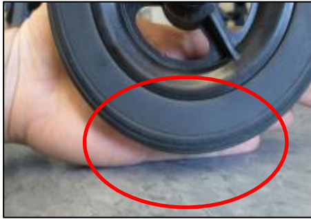
An example of a floating caster. Note the space between the bottom of the wheel and the ground. 18
