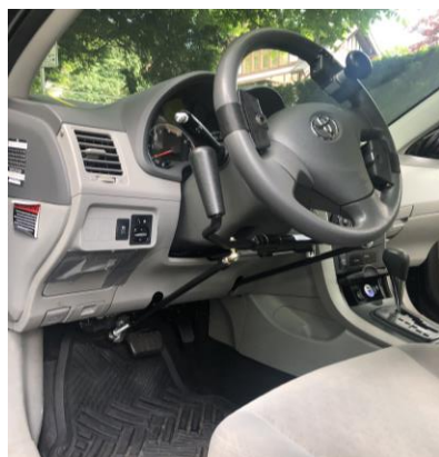
Rods can be connected to the accelerator and brakes to allow for hand control driving. 18
