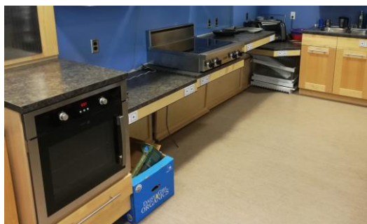
In the kitchen above, note the stove dials on the front of the stove and the space to wheel under counters. 9
