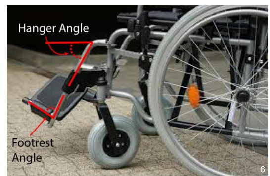
The footplate is angled away from the frame of the chair and the post of the casters. 6
