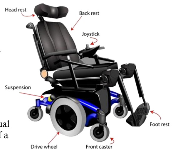
A typical power wheelchair includes a metal frame containing a motor and battery, a seat with a backrest, footrests, small caster wheels in the front and/or back, and two large rear wheels at the back. It is propelled and maneuvered using a joystick or other control function. 1
