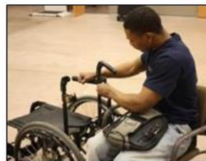
Inspect back posts and back support hardware
