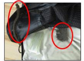
Cover foam liner flaking 14
