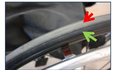
Intact (green) and worn out (red) tread on a wheelchair tire. 15
